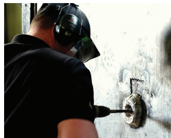
CYLINDER GUARD RESISTING DRILL ATTACK
