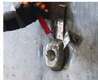
CYLINDER GUARD RESISTING WEDGE/PRY ATTACK
