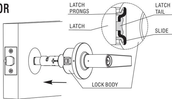
**3B:** Place lock body into position. Make sure that latch prongs engage chassis in housing, and slide engages latch tail.
