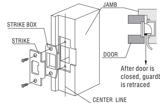
After door is closed, guardbolt is retracted
