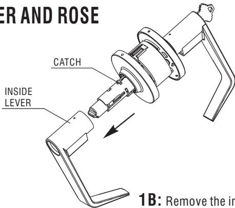
**1B:** Remove the inside lever from spindle.
