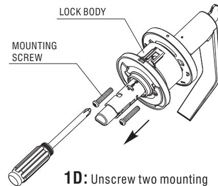
**1D:** Unscrew two mounting screws in lock body by screwdriver.
