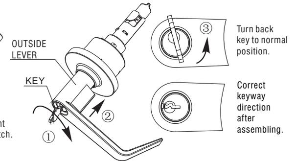
**2E:** Turn key 90° clockwise and push the lever into the maximum extent; rewind key.
