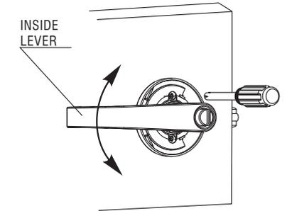
**3D:** Fix the inside lever and check if the rotation is smooth. Adjust the radial clearance between inside spring cage and inside lever.
