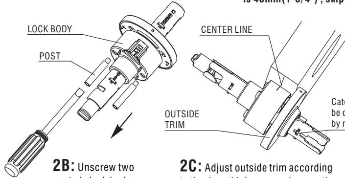
**2B:** Unscrew two posts in lock body by screwdriver.
