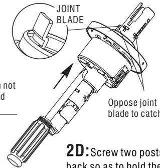
**2D:** Screw two posts back so as to hold the outside rose tightly.
