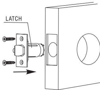
**3A:** Insert latch unit and fix it with two wood screws.
