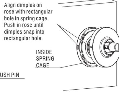
**3F:** Fix inside rose and make sure inside rose and inside spring cage are tightened.
