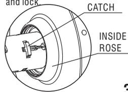
**3G:** Slide lever onto spindle. Push lever completely into place. (Pull on lever to make sure that catch is fully engaged).
