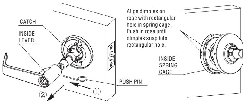
**3E:** Disassemble inside lever by push pin.
