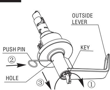
**2A:** Turn key 75° clockwise, insert push pin into hole in outside lever to depress catch. Remove the outside lever.
