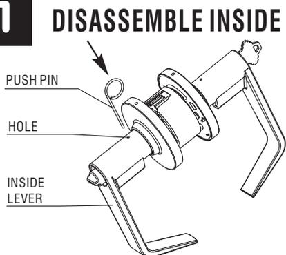
**1A:** Insert push pin into hole in inside lever to depress catch.
