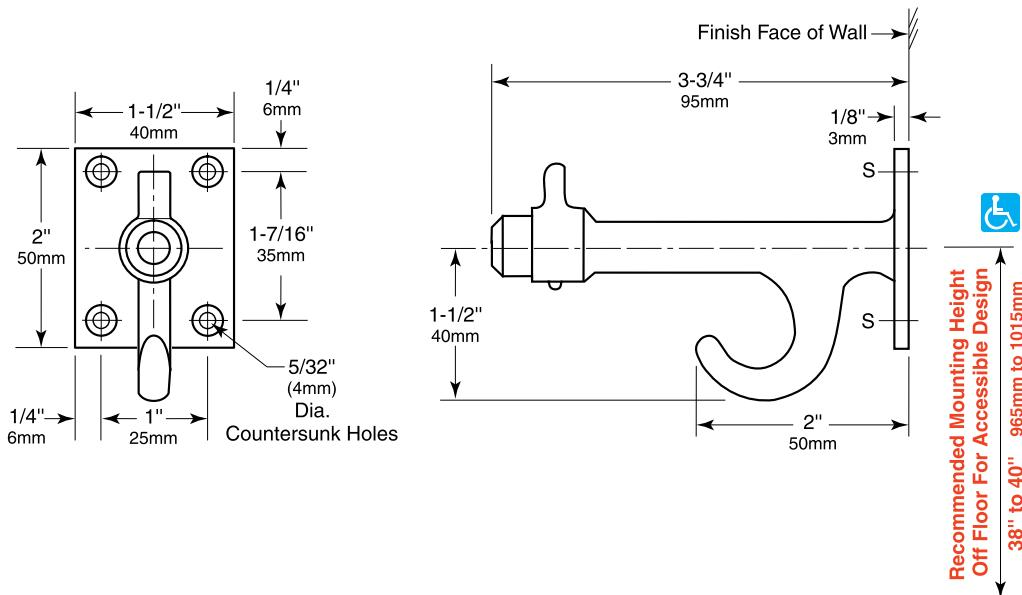
**MATERIALS:****Hook and Base** — Solid cast aluminum with matte finish.**Bumper** — Hard rubber secured with drive-screw. Protects wall or partition surfaces.**INSTALLATION:**
