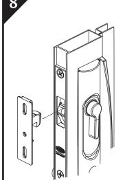
Insert striker into lock body to test operation.
