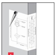
Position template and mark out drilling centres. Important also refer to lock manufacturer's template prior to drilling.
