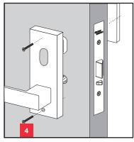
Insert spindle and spring supplied into lever to both sides of the door (spring locates fully into lever). Determine the correct screw length to suit the door thickness then cut screws
