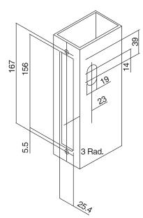
**1. Prepare Door** Cut opening in door to suit cover plate and drill holes to suit function required.
