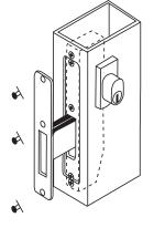
**3. Cover Plate** Attach cover plate to lock with 3 countersunk head screws (5mm long) supplied.
