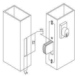
**4. Cut Bolt Hole** Cut a bolt hole in door jamb as shown.
