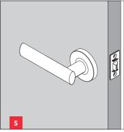
5. Install furniture to the door do not tighten screws with excessive tension on power driver as this may damage screws and void warranty. Screw on outer roses to lever set to complete installation.
