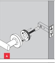
4. Insert spindle and spring supplied with levers to both sides of the door, as shown.
