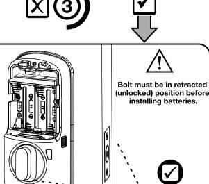
6 Installing Batteries/Handing the Lock
