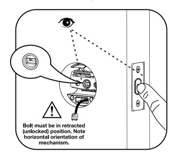
Installing Interior Mounting Plate
