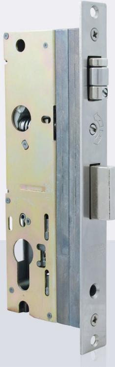
The Lockwood Optimum Roller Bolt Mortice Lock is designed to suit a wide range of door sizes for both timber and aluminium residential doors. The design allows for optimal latch adjustment and provides positive latching.
