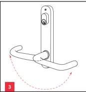
**3.** Non handed levers To change handing rotate lever 180°.
