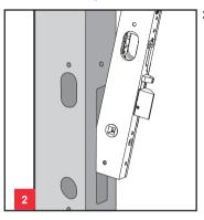
2. Important do not attempt to drill holes whilst lock is in mortice. Drill the 4.5mm fixing holes half way through the door and repeat on the other side, with the holes meeting in the middle of the door. Drill other holes that are required to match function of plates.
