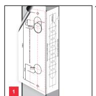
This template applies to bolt through fix lock/latch with a 23mm backset.
