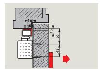
**Angle bracket for G-N**For push-side fixing of the slide channel to door frames with a deep reveal.
