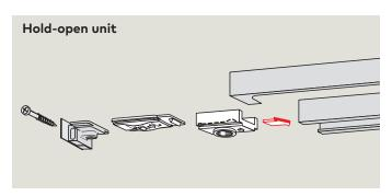
The **RF** mechanical hold-open unit ensures that doors are held open at precisely the correct angle – up to approx. 150° – without any fallback.
