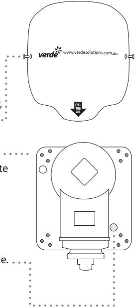
NOTE Hardwiring requires removal of plastic disc to expose thread hole. ....
