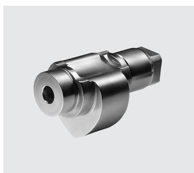
The heart-shaped cam and the linear drive mechanism of the TS 90 Impulse ensure that the resistance encountered decreases almost instantly with the door opening action – so even children, the elderly and people with disabilities have no problem in opening the door.
