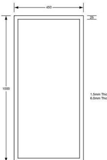
1.5mm Thick Frame Profile 6.0mm Thick Safety Glass
